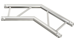
135° 2WAY C23 H CODE G32C23H L050 W500 H500(mm)
